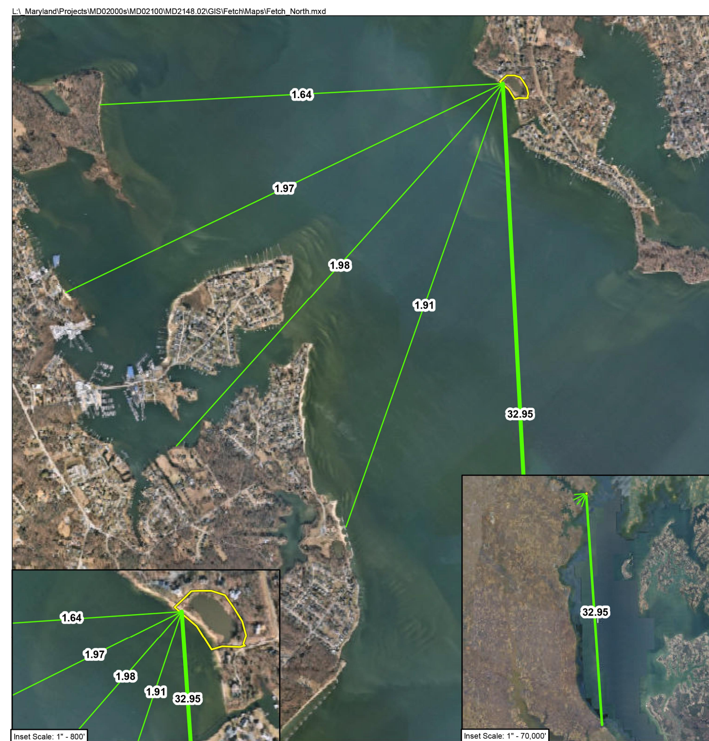
Site Fetch Map - North Southbreeze Shoreline Stabilization WSSI #MD2148.02 Legend: Site (Yellow) Fetch - Component of Average (mi.) (Green) Fetch - Longest and Component of Average (mi.) (Purple) Scale: 1" = 2,000' NORTH
