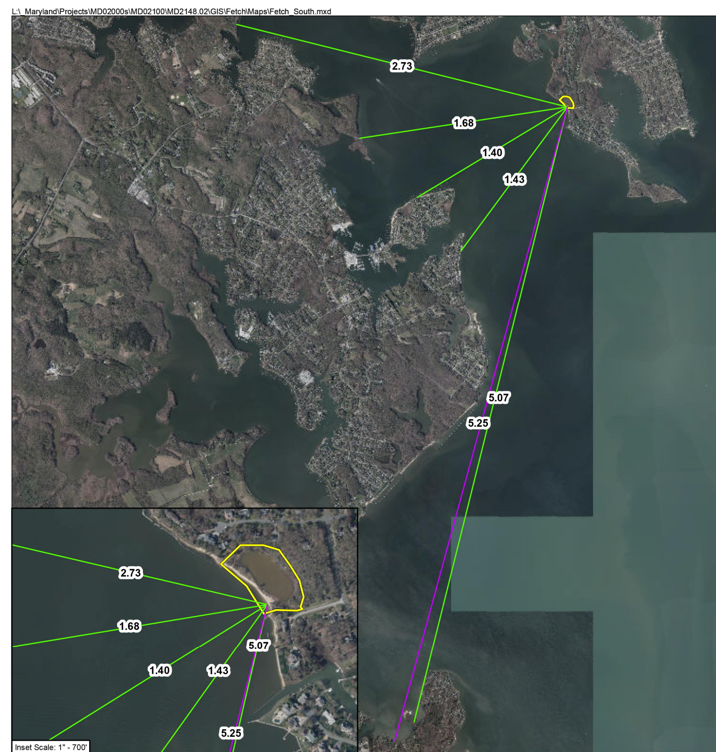
Site Fetch Map - South Southbreeze Shoreline Stabilization WSSI #MD2148.02 Legend: Site (Yellow) Fetch - Component of Average (mi.) (Green) Fetch - Longest and Component of Average (mi.) (Purple) Scale: 1" = 4,000' NORTH
